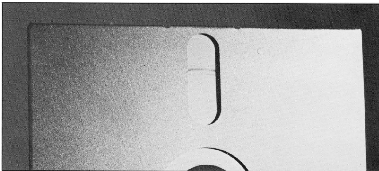
Figure 3-8. Defective 5 1/4-inch Flexible Disc
